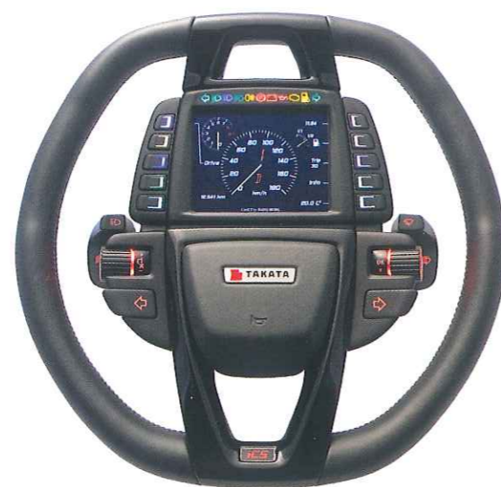
4 Driveable prototype of the iCS interactive steering wheel with fully integrated display which has a touch function and is positioned at the same level as the conventional instrument cluster
